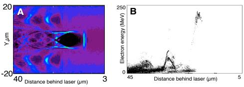
**FIGURE 4.** Simulations show that beam loading and pulse evolution turn off injection after the trapping of an initial bunch, resulting in a bunch isolated in phase space. This is visible in the density contour (A), where the wake amplitude is lowered following the bunch in the first bucket. The particles are then concentrated in energy at the dephasing length (B).
